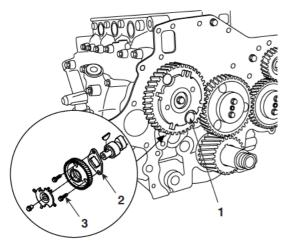
6. Install the supply pump gear.
