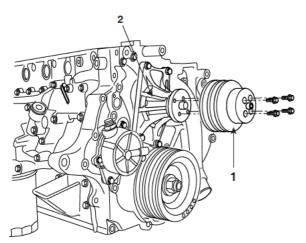
4. Remove the vacuum pump (1) and alternator assembly (2).
