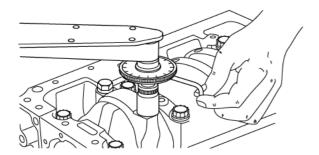
Remove the connecting rod bearing cap and measure the oil gap at each pin journal.
