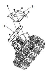
Remove the turbocharger assembly (1) from the cylinder head.
